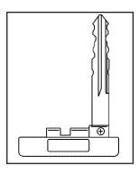
This key, located inside the keyless access transmitter, can be used for the driver's door, glove box, and rear seat pass-through door. See "Rear Seat Pass-Through Door" under *Trunk on page 101* for more information.
